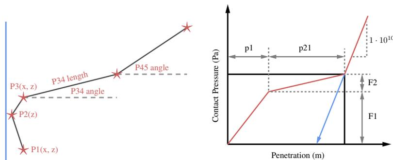
**Fig. 1.** Vehicle geometry and stiffness design variables
